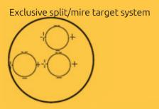
Keratometer II's internal measuring scales
